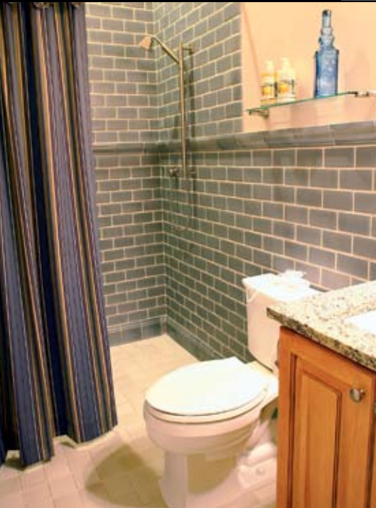
Roll-in showers with non-slip surfaces are safe for disabled or elderly homeowners using walkers or wheelchairs.
